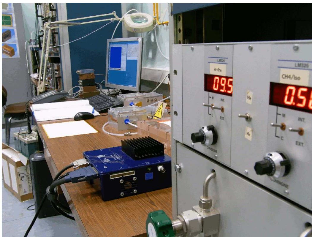
Figure 30. Saclay laboratory setup: NIM rack with HV (background), computer with Pixelman software, InGrid storage box, experiment box, Micromegas box, MUROS interface (see section 3.3) and gas mixer (in the front).
