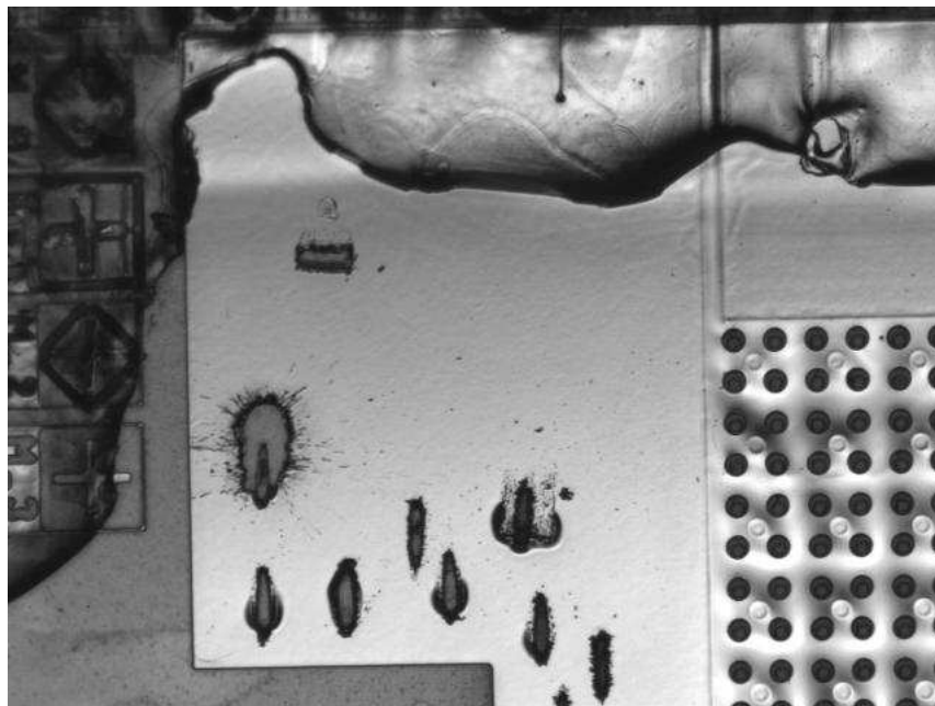
Figure 28. Microscope image of the bonding pad of the grid on chip G06-W0096. The big hole on the pad on the left was the place where a wire bond was fixed. The other holes come from several attempts of bonding.
