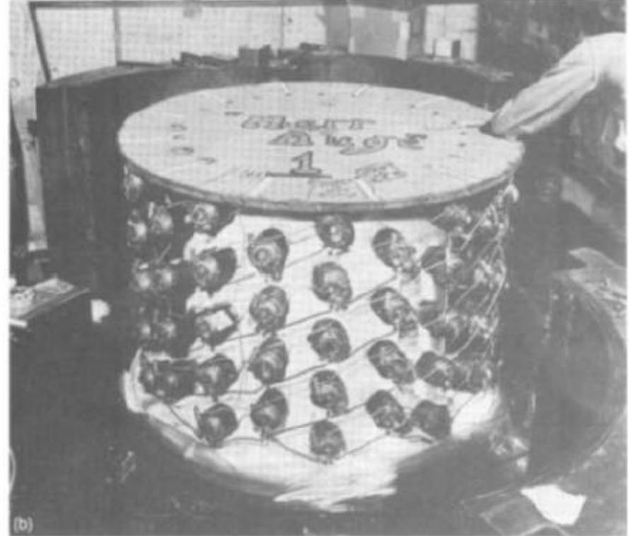
The detector itself - a 300-litre tank of liquid scintillator, surrounded by 90 phototubes. Before this, 20 litres of liquid had seemed a large volume!
