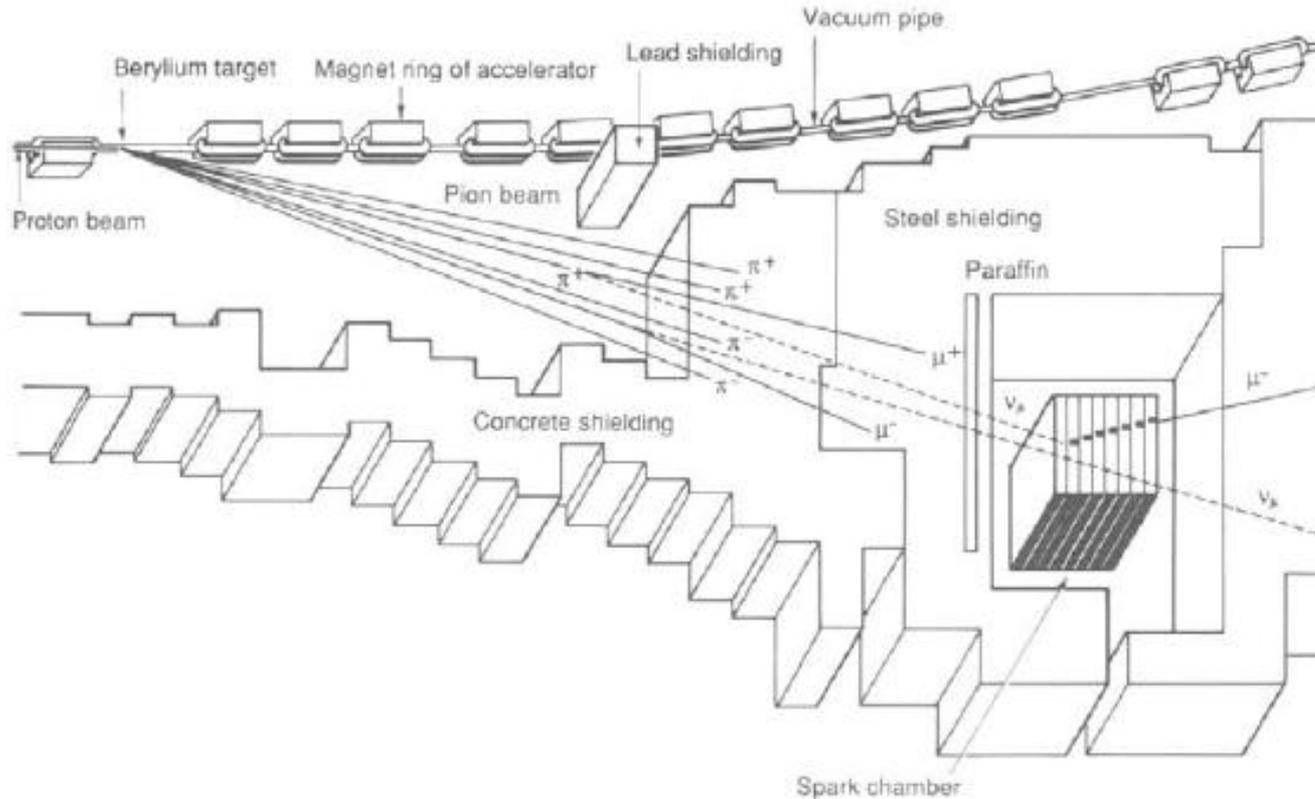
The principle of the first high-energy neutrino experiment at Brookhaven was to create the neutrinos in the decays of pions produced when protons in the accelerator struck a target of beryllium. Large amounts of steel shielding in a wall 13.5 meters thick absorbed both the muons produced and the remaining pions, allowing only the neutrinos to penetrate to the 10-tonne spark chamber.
