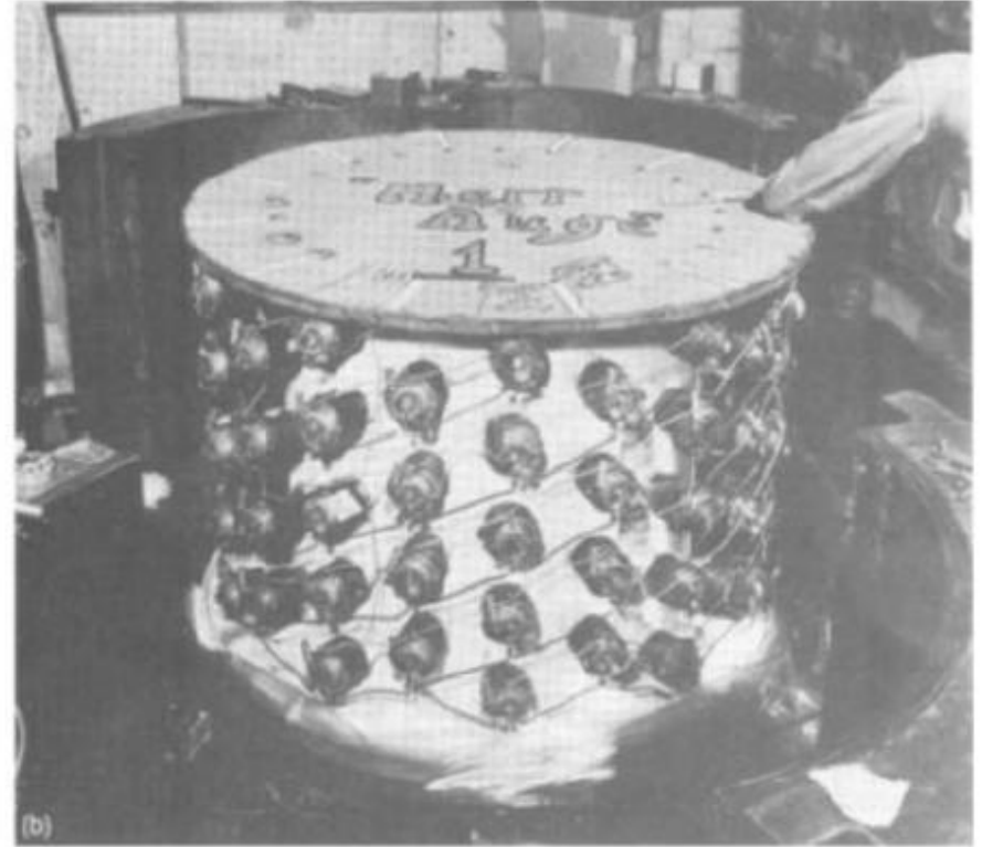
The detector itself - a 300-litre tank of liquid scintillator, surrounded by 90 phototubes. Before this, 20 litres of liquid had seemed a large volume! (Los Alamos National Laboratory)
